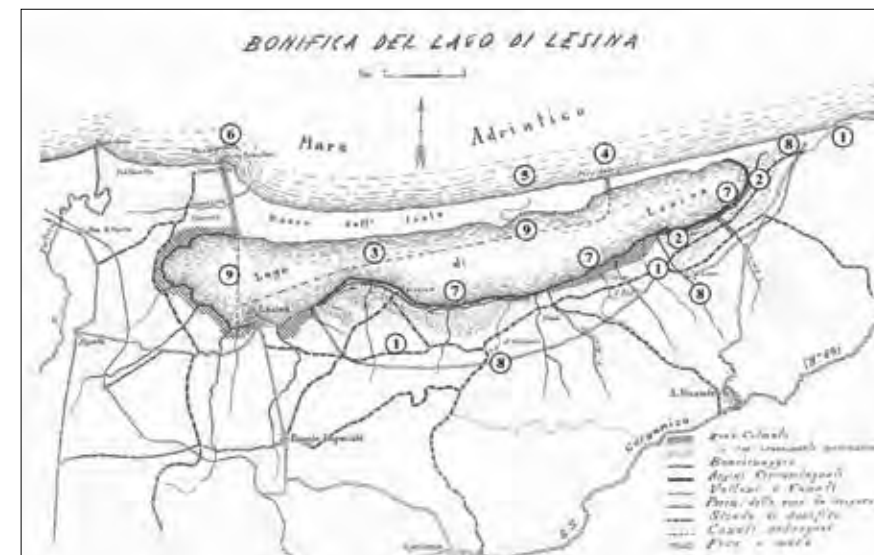
KEY: 1. Lesina-Rodi Road 7. Dikes 2. Eastern wetlands 8. S. Nazario Springs and Longo River (left to right) 3. 1811 division 9. Sub-alluvial canal. 4. Schiapparo Channel 5. S. Andrea Channel 6. Acquarotta Channel
