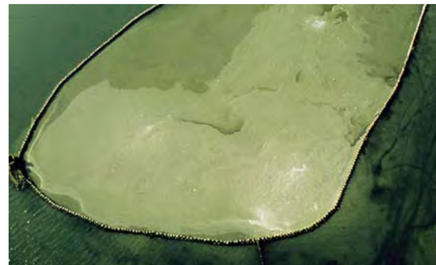
Figure 9: artificial salt marsh: cordoned off area filled with materials resulting from diggings.
