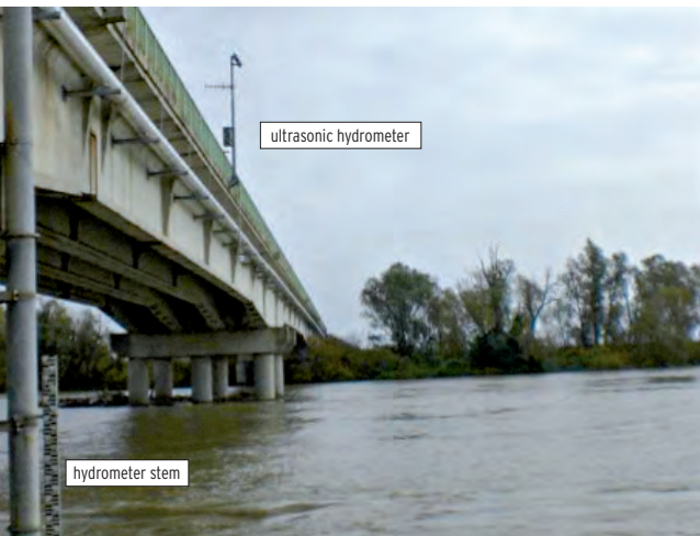
Figure 2b: view of hydrometric monitoring installation (hydrometer stem and ultrasonic hydrometer) on the Po di Gnocca.
