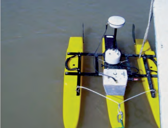
Figure 2a: ADCP sensor towed by boat used for conducting flow rate measurements.
